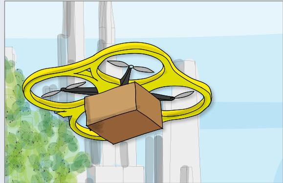
**Drones.** Autonomous aircrafts, e.g., copters or vertically starting planes, carry parcels (up to 15 kg) to their destination along the most direct route and at relatively high average speed. Like droids and AGVs, they too need to be supervised. We believe that one supervisor per roughly eight drones is a reasonable assumption.
