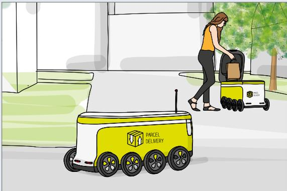
**Droids.** Small autonomous vehicles, only slightly larger than a regular parcel, deliver parcels to the doorstep. These vehicles are relatively slow at 5 to 10 km/h and use the sidewalk rather than the street to reach their destination. Such droids also need to be supervised, but due to their size and low speed, developers currently believe that a single supervisor could manage 50 to 100 of them.
