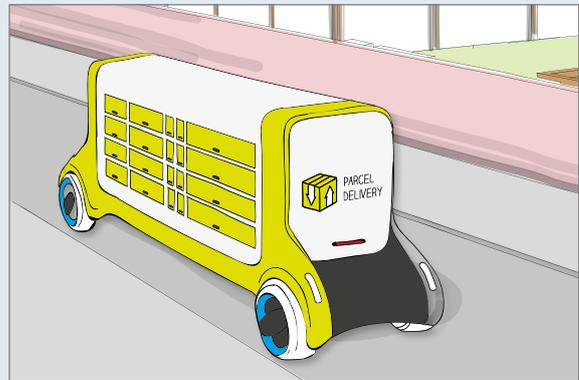
**Autonomous ground vehicles (AGVs) with lockers.** AGVs deliver parcels without any human intervention. Customers are notified of the exact arrival time. Upon arrival at their door, customers are asked to pick up the parcel from the specified locker mounted on the van or truck – picture a mobile parcel locker. Granted, such vehicles would need to be supervised. We assume that a central supervisor could manage roughly eight to ten AGVs.
